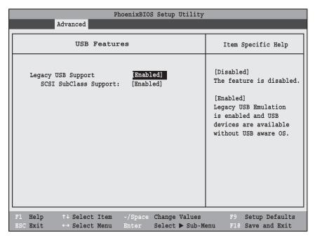
Figure 9. USB Features Submenu
